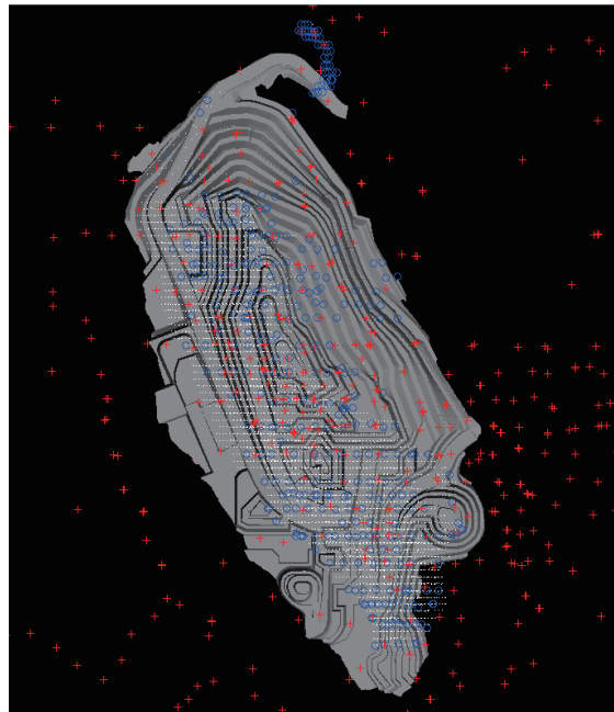
Figure 7: Plan showing distribution of GC (white dot), RC (blue circle) and DD (red cross) collar locations. Preliminary pit design as at December 2015.
