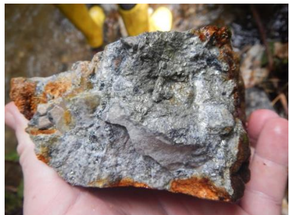
Photo 12. Macro of the silica-pyrite-chalcopyrite veinlets present in the outcrop pictured left. Note the blue-black secondary Cu oxide mineralization after chalcopyrite.
