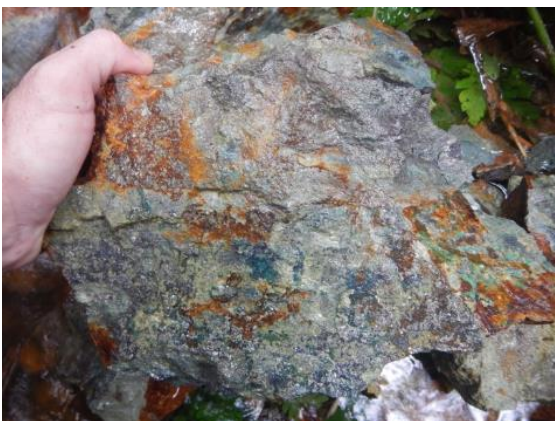
Photo 23. Cu stained and Cu oxide bearing diopside, magnetite, epidote, chlorite skarn. Contains abundant disseminated pyrite-chalcopyrite mineralization.
