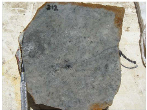
Photo 10. Tonalite pictured left hosting texturally destructive alteration and quartz – kspar – pyrite - chalcopyrite veinlets with secondary Cu oxide (blue-black mineral, center).
