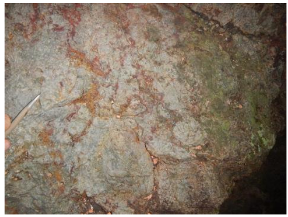
Photo 14. Silica, sericite and tourmaline replaced microdiorite cut by quartz-pyrite +/-chalcopyrite sealed crackle breccia, from outcrop pictured left (Photo 9).
