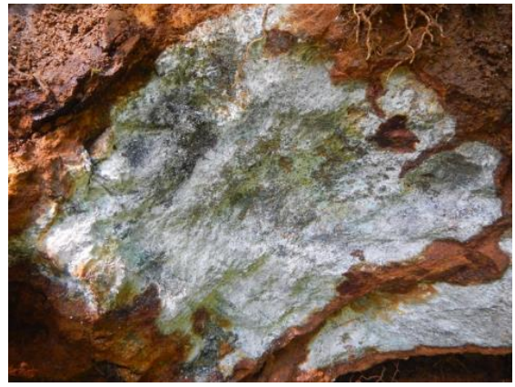
Photo 20. Altered silty sandstone pictured left, containing abundant disseminated pyrite-chalcopyrite and secondary Cu oxide mineralization (blue-black).
