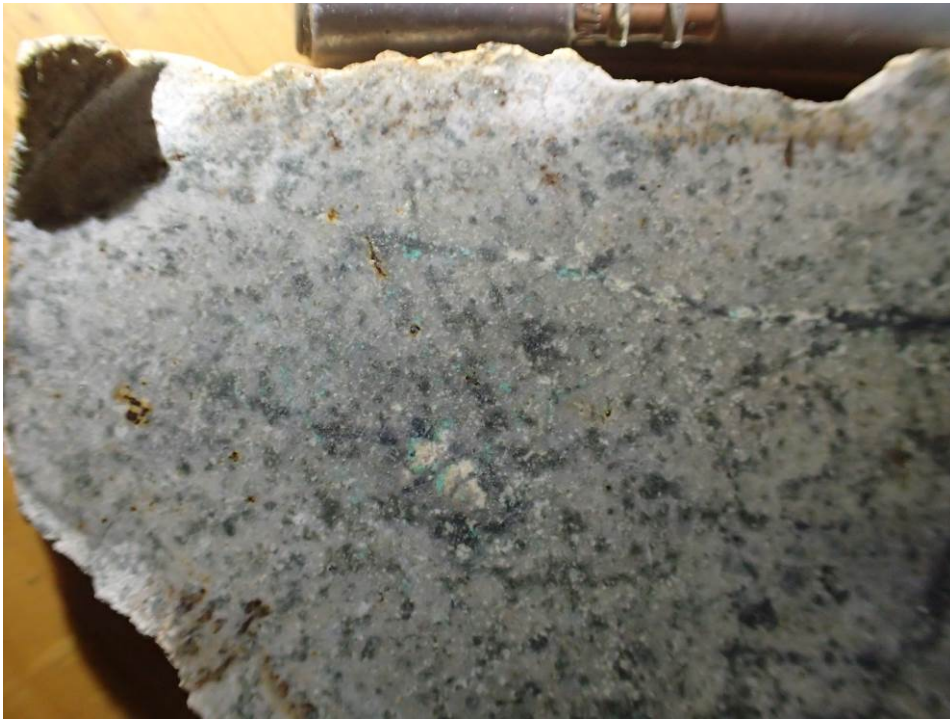
Vein hosted and disseminated chalcopyrite (here allowed to oxidize after cutting to green malachite, for better visibility within this photograph). The host rock is altered diorite. Cross cutting veins are composed of quartz-magnetite-pyrite-chalcopyrite. The width of this photograph is approximately 8 cm.
