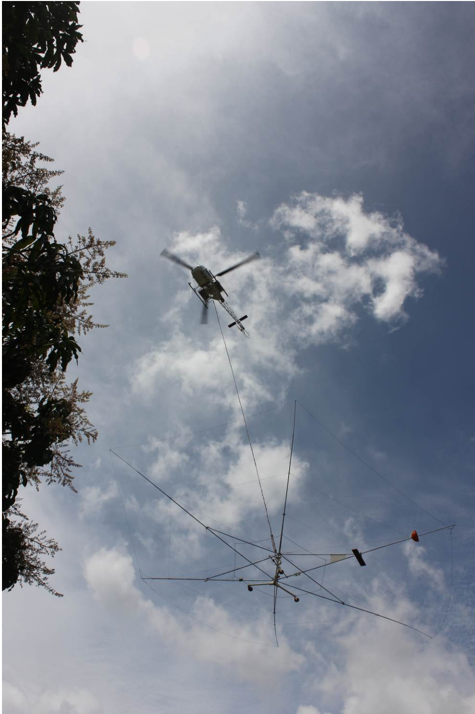
The heli-borne Electromagnetic survey in operation at the Rantau Panjang area.
