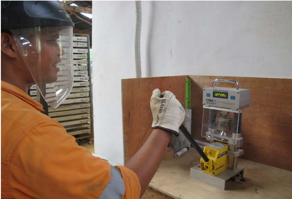
A core shed assistant operating a point load index testing machine on core from the Tor Uluala deposit. This machine tests the in-situ rock strength which is used for estimating process plant crushing and grinding characteristics, pit wall strength and blasting requirements.
