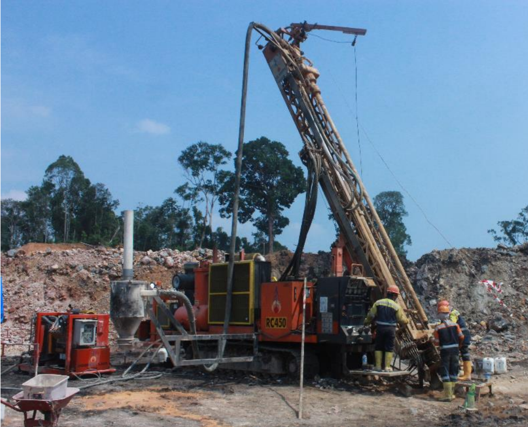
RC drilling in the Purnama open pit. This is the second RC rig on site, dedicated to resource development drilling. It is currently drilling infill delineation holes to greater than 100m depth.
